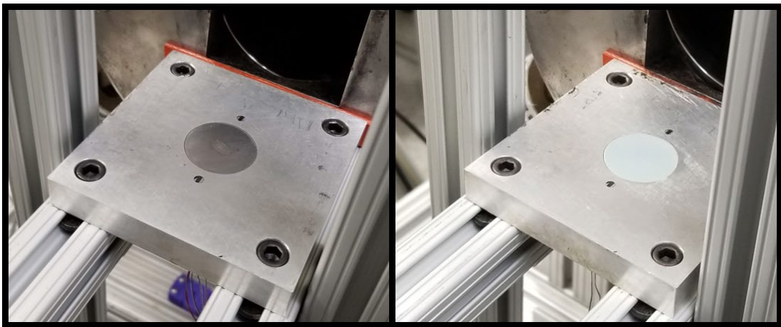
Figure 20: Comparison of Unpainted (left) vs. Painted (right) Test article plate
